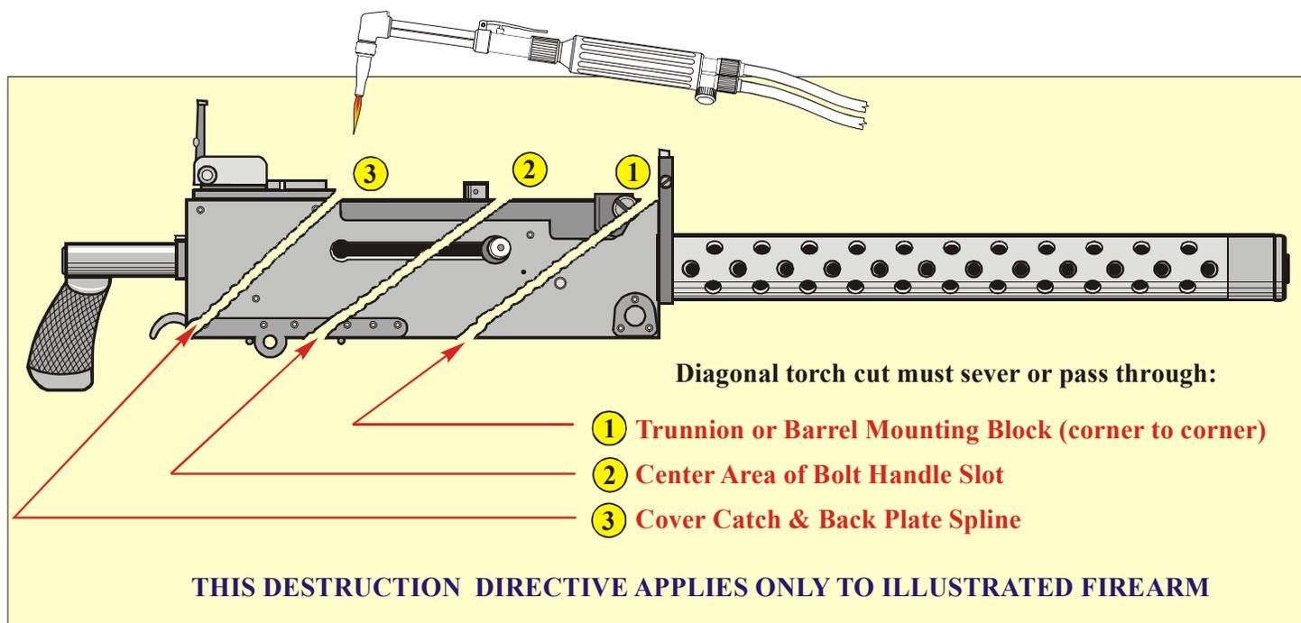
The purpose of this procedure is to destroy the receiver or frame in a manner that will prevent its function and future use as a firearm. A proper method of destroying this firearm is to cut the receiver into separate pieces as follows:
