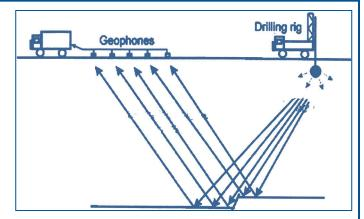
Seismic field operations typically involve at least three distinct entities: An explosives company (supplier), a shot hole drilling company, and the seismic company that ultimately detonates the explosives and records geophysical data. Each of these entities has certain licensing and operating requirements under the Federal explosives regulations at 27 CFR, Part 555.
