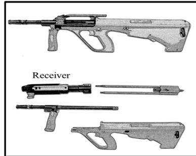
(vii) *Thompson M1A1-type machineguns and semiautomatic variants, and L1A1, FN FAL, FN FNC, MP38, MP 40, and SIG 550-type firearms, and HK-type machineguns and semiautomatic variants*: the upper part of the weapon that provides housing for the bolt and firing pin.
